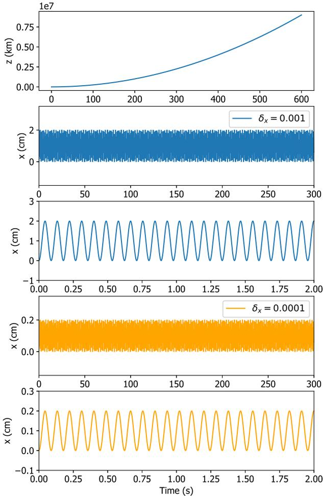
Figure 5: Spacecraft position for small initial perturbations in  $X$  and  $\theta_y$ . Simulation results.
