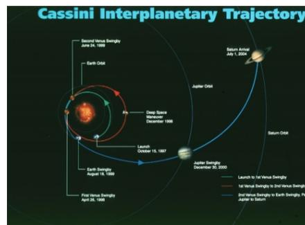
Fig1. Cassini Interplanetary Trajectory
