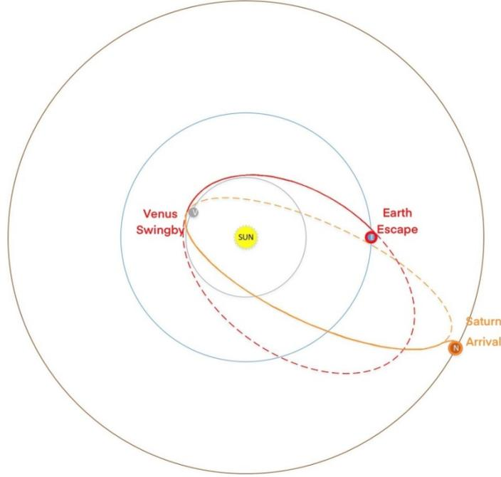
Fig2. Schematic diagram of voyage trajectory
